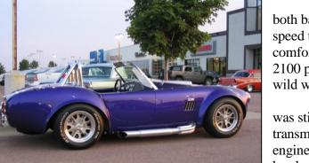
"The traction-lok rear-end has 373 gears keeping both back tires locked on quick take-offs and the fivespeed transmission offers a top speed beyond my comfort level," Clay said. "The total car weighs only 2100 pounds so the power to weight ratio really makes it wild when the second carburetor comes out to play."
