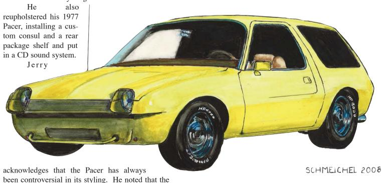
passenger door is four inches longer than the driver's door to make it easier for people to access the back seat.
