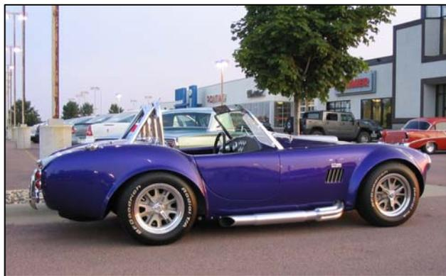
"The traction-lok rear-end has 373 gears keeping both back tires locked on quick take-offs and the five-speed transmission offers a top speed beyond my comfort level," Clay said. "The total car weighs only 2100 pounds so the power to weight ratio really makes it wild when the second carburetor comes out to play."
