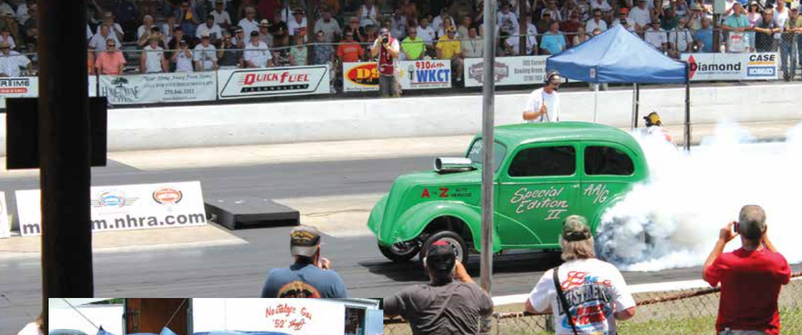
“Boiling the hides” for the fans at Beech Bend Raceway is an AA/ Gas Anglia (an English Ford). Smoky burnouts like this heat the slicks for maximum traction on the start.
